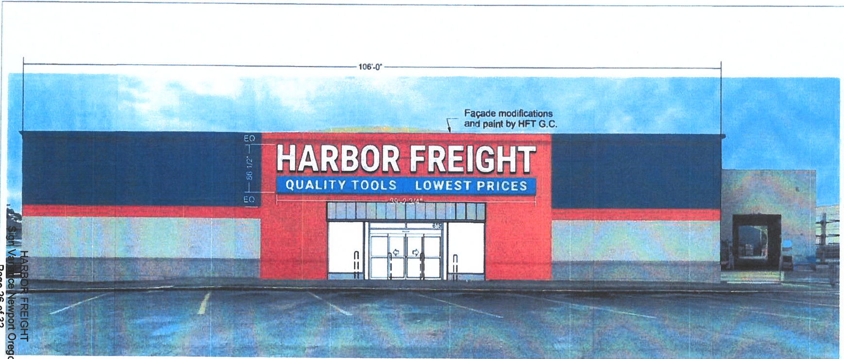
FRONT ELEVATION - Sign Type (A) (QTY:1) Channel Letters on Raceway Scale: 3/32" = 1'-0" (282.78 sqft)
