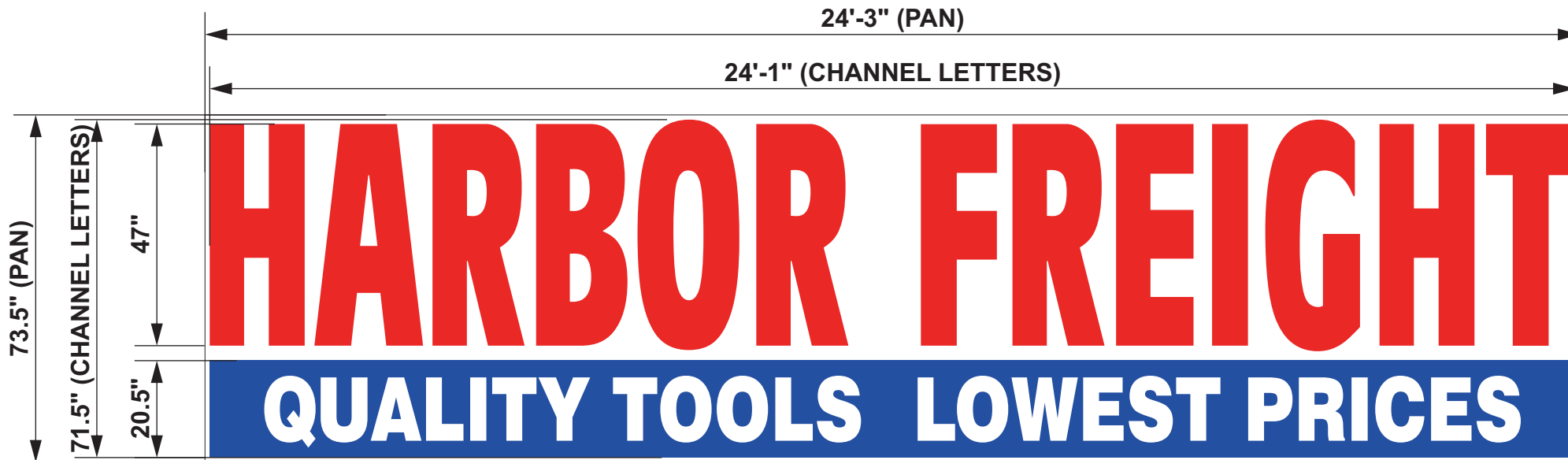
Front Elevation - Sign Type (A) (QTY: 1) Channel Letters - Pan Mounted Scale: 3/8" = 1' (148.5 SQ FT)
