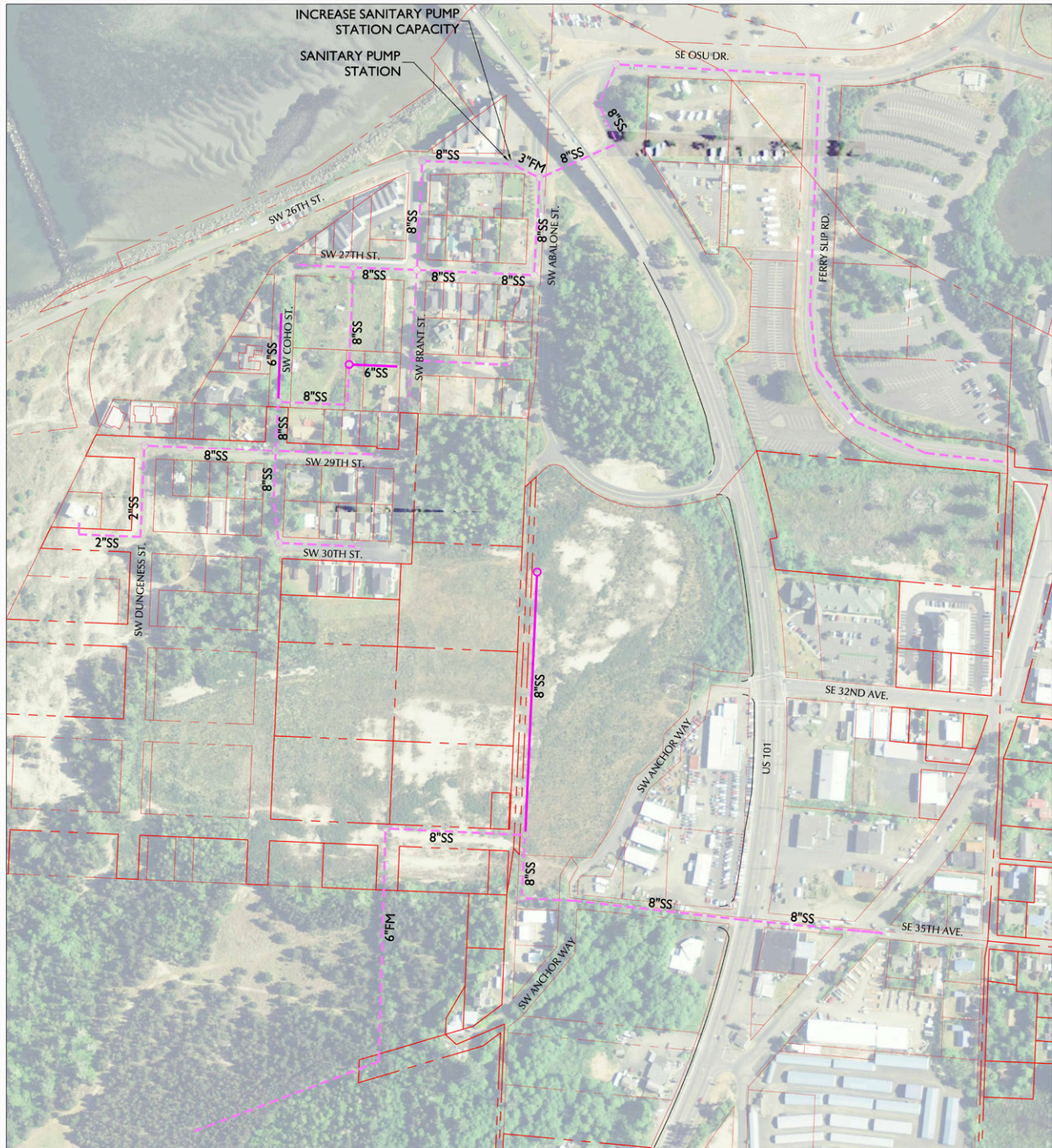
Map 3-6. Proposed Sanitary Sewer System Improvements
