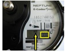
These meters will be installed over time. It will alternately flash a "USE" and "RATE" window. If all water is off, anything over 0.00 in the "RATE" window means a leak.
