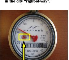
That red triangle will turn if any water is flowing through the meter. If all the water is off and it's turning, you probably have a leak.
