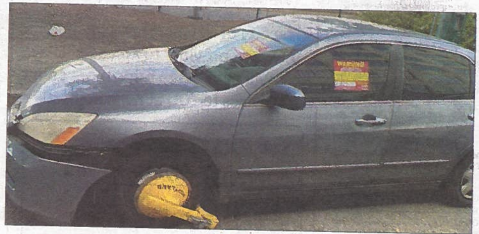
Immobilizing a vehicle includes use of a mechanical tool called a boot that locks the vehicle in place. (Courtesy from the City of Portland)
