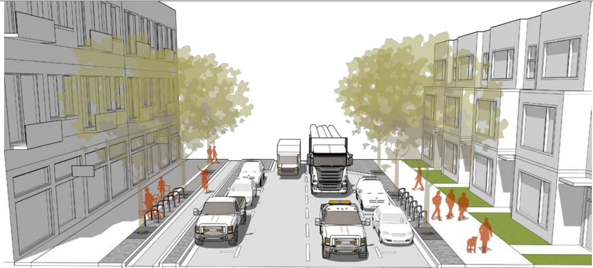
Cross Section illustrates Urban Frontage – Shopfront (left) and Urban Frontage – Residential Porch-Stoop-Terrace , (right), see page 40.
