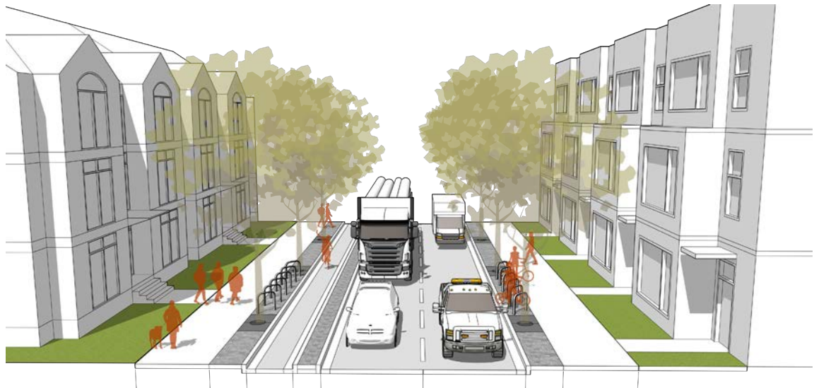
Cross Section illustrates Urban Frontage – Residential Porch-Stoop-Terrace , vertical separation standard (left); horizontal separation standard (right), see page 40.
