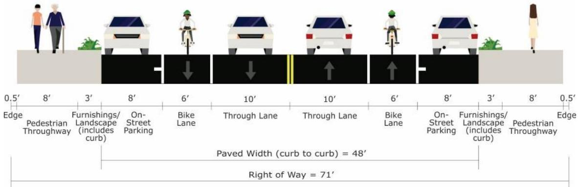
**FIGURE 31: CITY MAJOR COLLECTOR (NON-COMMERCIAL AREA) CROSS-SECTION**
