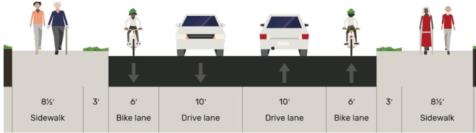
**FIGURE 34: ACCEPTABLE NEIGHBORHOOD COLLECTOR TYPICAL CROSS-SECTION**
