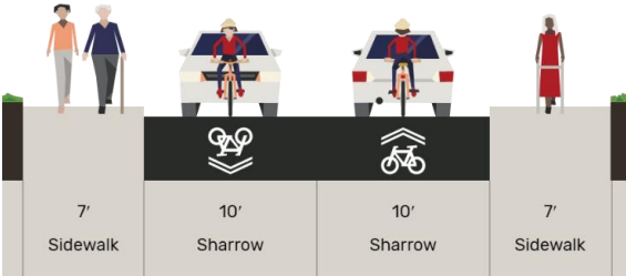
FIGURE 12A: ACCEPTABLE LOCAL STREET TYPICAL CROSS-SECTION – PARKING ONE SIDE ONLY (SOURCE: STREETMIX)
