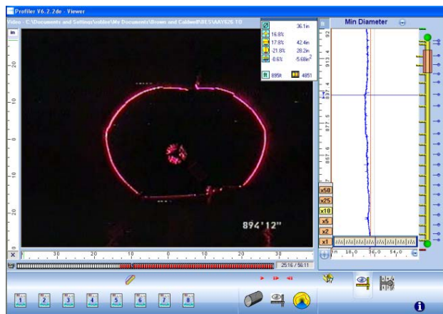
Figure D-12. Laser projection from laser profile inspection
