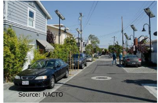
Shared street example with intermittent on-street parking.
