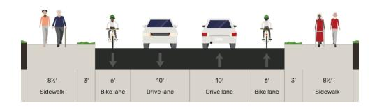
FIGURE 34: ACCEPTABLE NEIGHBORHOOD COLLECTOR TYPICAL CROSS-SECTION
